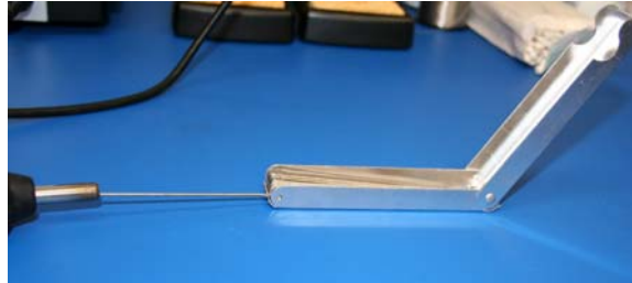
Figure 8: Using the Desoldering Iron Cleaning Tool
