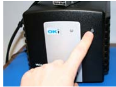
Figure 24: Power Button on the OKI Soldering Station
