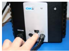
Figure 25: Select the Soldering Iron on the OKI Soldering Station
