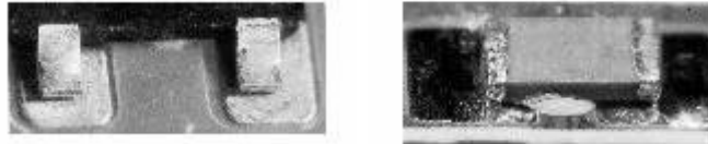
Figure 44: SMT Examples with Too Little Solder Used
