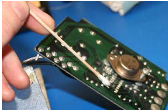
Figure 36: Re-Clean the Desoldering Area
