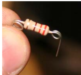
Figure 17: Coiled Resistor Leads to Reduce Vibration Shearing
