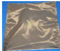
Figure 32: Use an Antistatic Bag for all PCB Transportation and Storing
