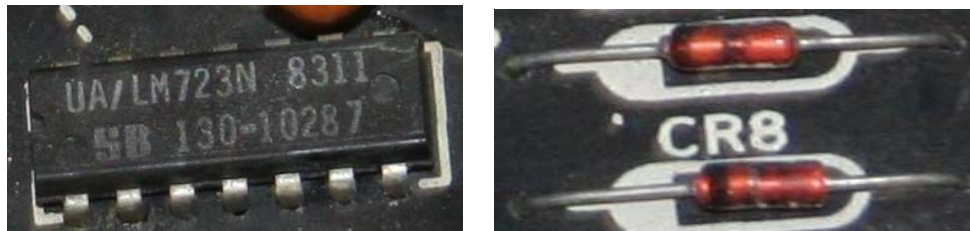
Figure 4: Example of DIP16 and DO-35 Packages
