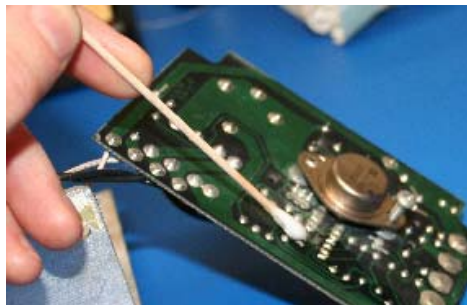
Figure 23: Re-Clean the Desoldering Area
