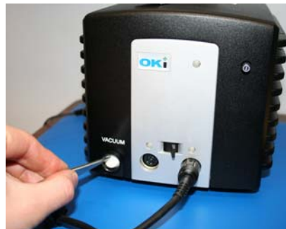
Figure 8: Changing the Filter in the Desoldering Iron
