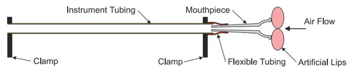
**Figure 8: Schematic diagram of the simple brass instrument with flexible tubing to decouple the lips from the instrument's walls**
