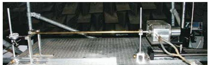
Figure 3: Simple brass instrument being blown by artificial mouth
