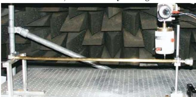
Figure 1: Simple brass instrument being mechanically driven by the shaker
