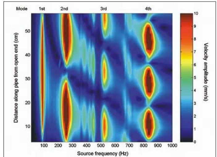
Figure 2: Velocity amplitude variation as function of frequency along the simple brass instrument when driven by a mechanical shaker
